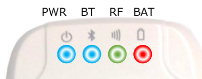
図 8-8 Dragon_BLE の LED 配置
